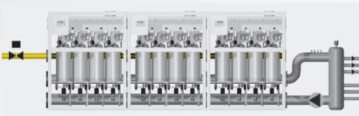
Example of a cascade installation of a total of 600 kW with inverse return.
